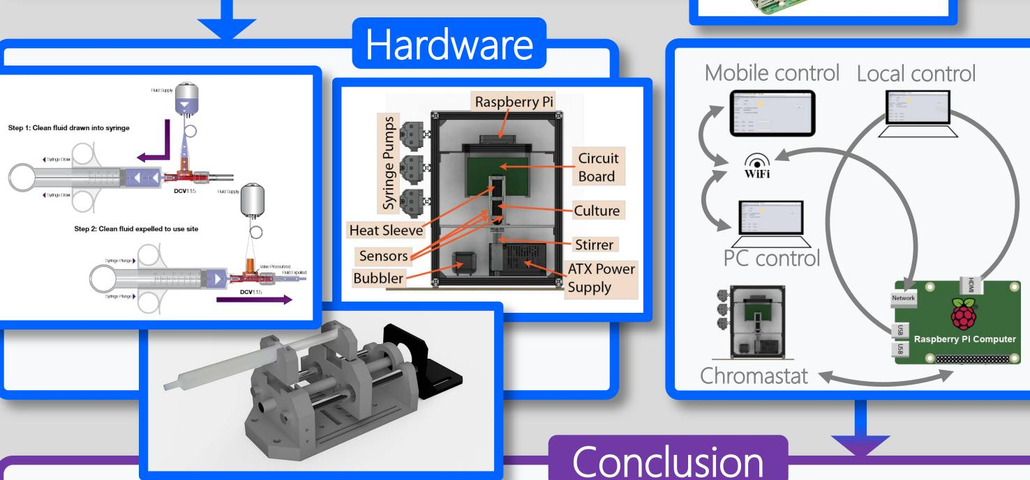
Our project can measure metabolites in the violacein pathway using an RGB sensor and autonomously regulate gene expression by varying inducer input. This proof of concept is modular; any part of this can be switched with another part or combined with additional parts so that it is customizable for both research and industry.
