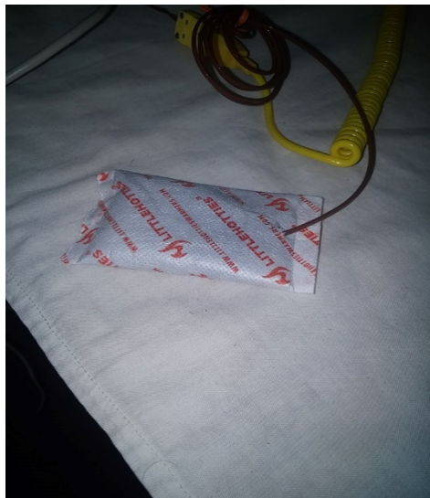
Figure 2. The thermocouple is exposed to the chemical inside the hand-warmer.
