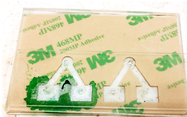
Figure 16. Bifurcated chip design with 2-3mm inlet holes and a total of 4 rectangular reaction chambers. The chip had 3mm wide fluid channels linking the inlets and the reaction chambers. Notice the green dye being absorbed into the surrounding paper backing.
