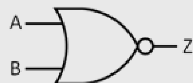
Figure 1. Schematic of a NOR composition showing input A, B and output Z.
