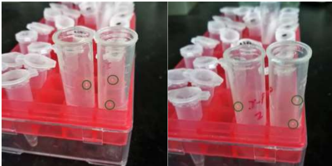
(Fig.1 The parts surrounded by dark green circles are dry powder. The protective reagent is glycerol.)
