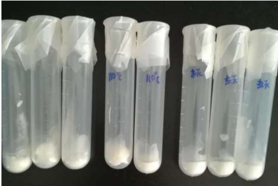
(Fig.2 The protective reagent of 3 groups on the right and left is without any treatment. The reagent of 2 groups in the middle is sterilized at 115^{\circ}\text{C} for 15 minutes.)
