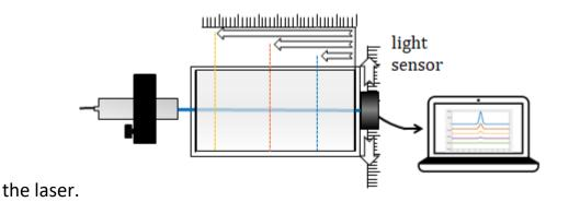
To reduce the path length of the laser within the gel, the measurements were repeated with different lengths of gels.
