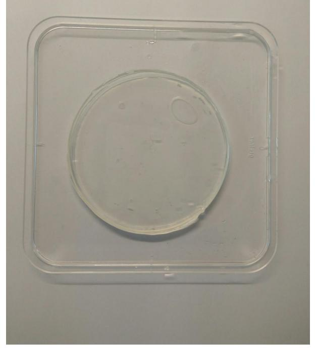
20.09 Setting low concentration Alginate on top CaCl2 agar: <u>Goal:</u> as previous experiments showed that 0.5%. Alginate produced strong gel when set overnight over agar, I tried with 0.25% and 0.1%:
