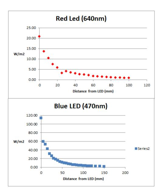
The blue and red light intensity needed are blue=2.8nm , red=11.1nm , therefore the distance from the LED must be blue=11-12cm, red=1-2cm
